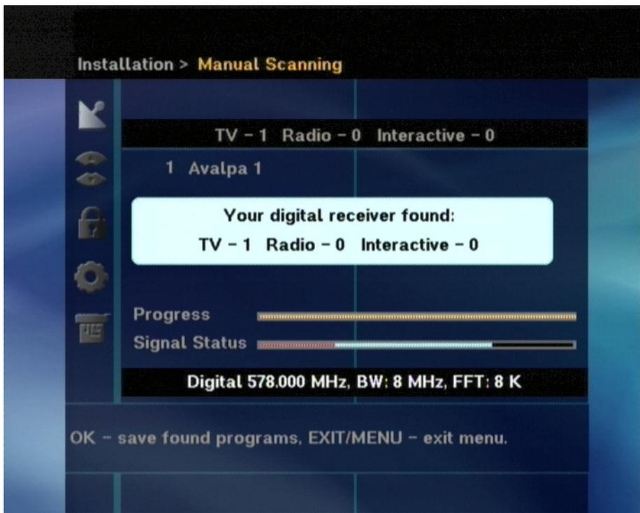
Check the modulation parameters that the decoder is using actually match the one from the command line, the signal status strength is also high.
